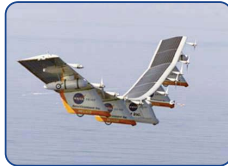
Figure 2-1. The Helios Prototype developed by AeroVironment and tested by NASA. A solar and fuel cell system-powered unmanned aerial vehicle
